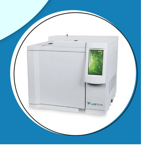
Gas Chromatography LGC-B11 is a benchtop unit with advanced flow controller (AFC) technology. System has digital control mode and polar capillary columns to separate polar analytes. GC oven is capable of 9 temperature program ramps and hold steps, and features rapid cooling: 250 °C to 50 °C < 10 minutes. Accurate flow rate control via AFC has higher level repeatability of retention time and peak area, enabling specific level of analysis by means of dual FID detectors.
